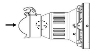
2. Align the lens alignment mark on the shade to the shade alignment mark on the objective lens and then push it in.
