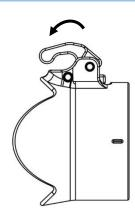
1. Make sure the locking lever is in open position.
