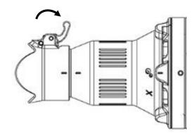
3. Lock the shade by pushing the locking lever downwards.
